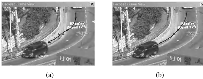
Fig. 7. Comparison of object tracking. (a) Object tracking in IPP encoded frame. (b) Object tracking in N-MV field.
